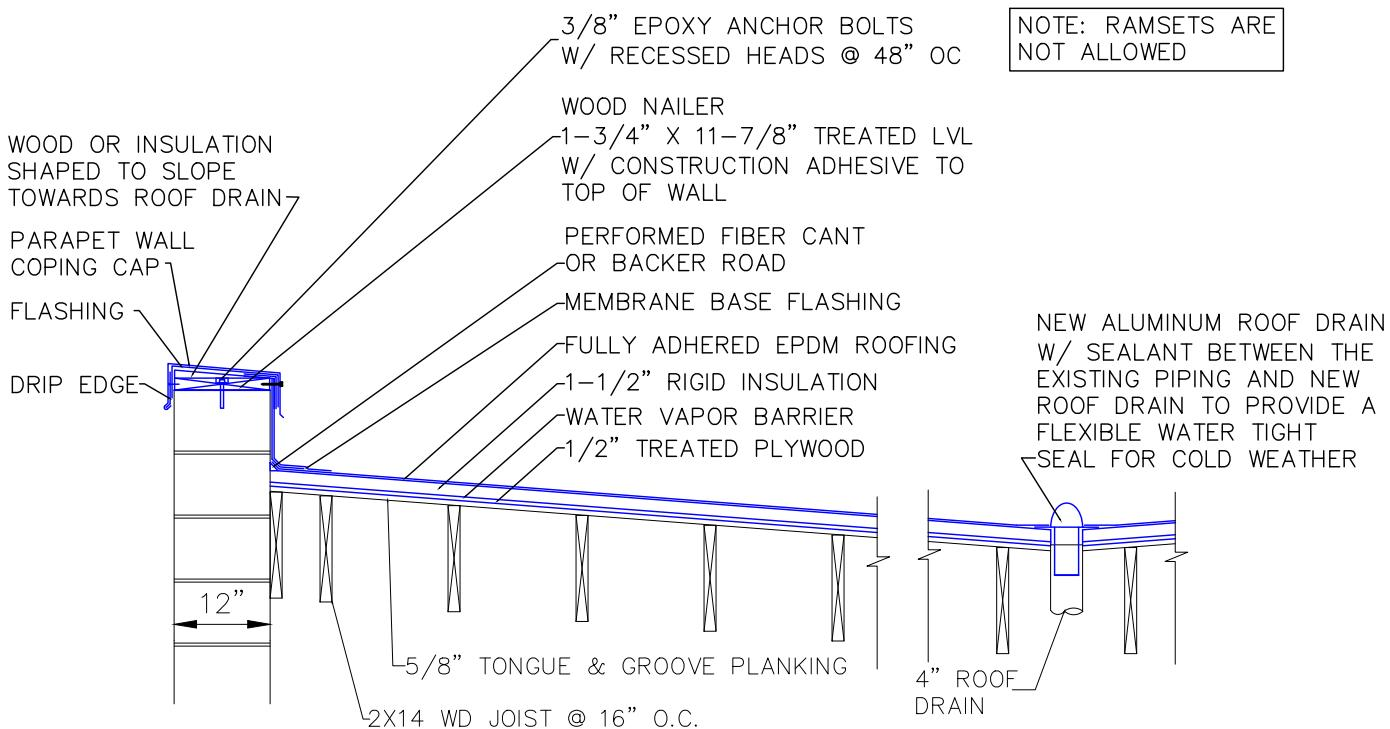
**PROPOSED ROOF SECTION PARAPET WALL DETAIL**
